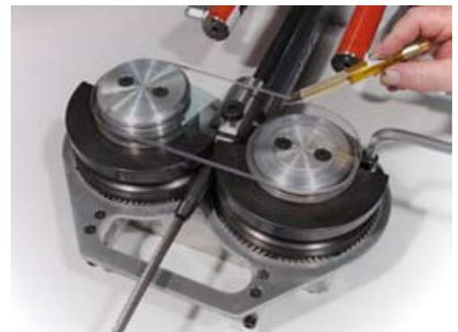
**4** Move the transparent protective shield into position. Apply hydraulic pressure to draw the terminal between the roller dies.
