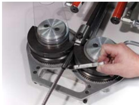
**3** Apply just enough hydraulic pressure so that the roller dies holds the terminal firmly. Then mark and insert the cable into the bottom of the terminal throat.
