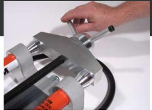
**2** Attach the terminal to the attachment fixture on the drawbar, and adjust the length so the roller dies meet the terminal shank at desired position.
