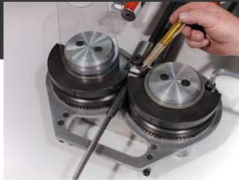
**1** Choose the pair of roller dies that corresponds to the cable diameter, and slip them onto the cogwheel synchronizing pins. The arrows on the dies should always be in the swaging direction.
