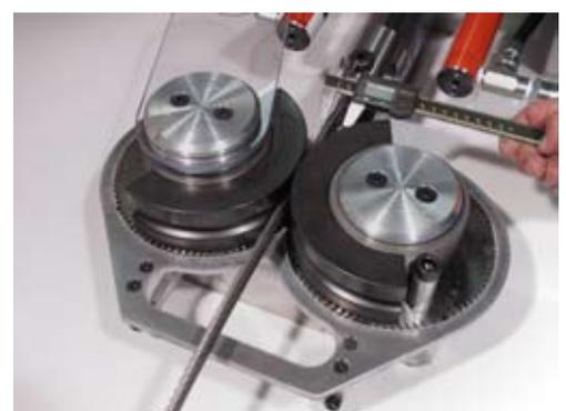
**6** Measure the diameter of the terminal after swaging, and compare with the swage dimensions list.
